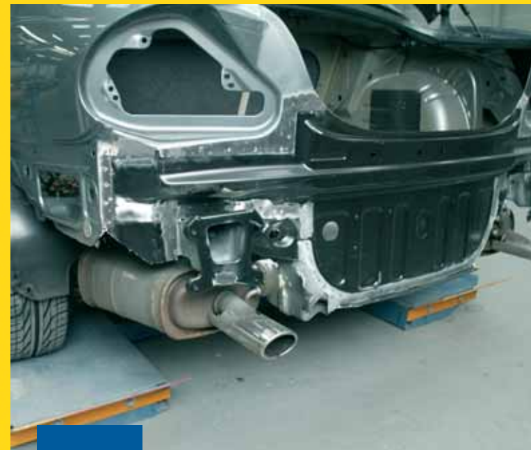
8 New welded part
