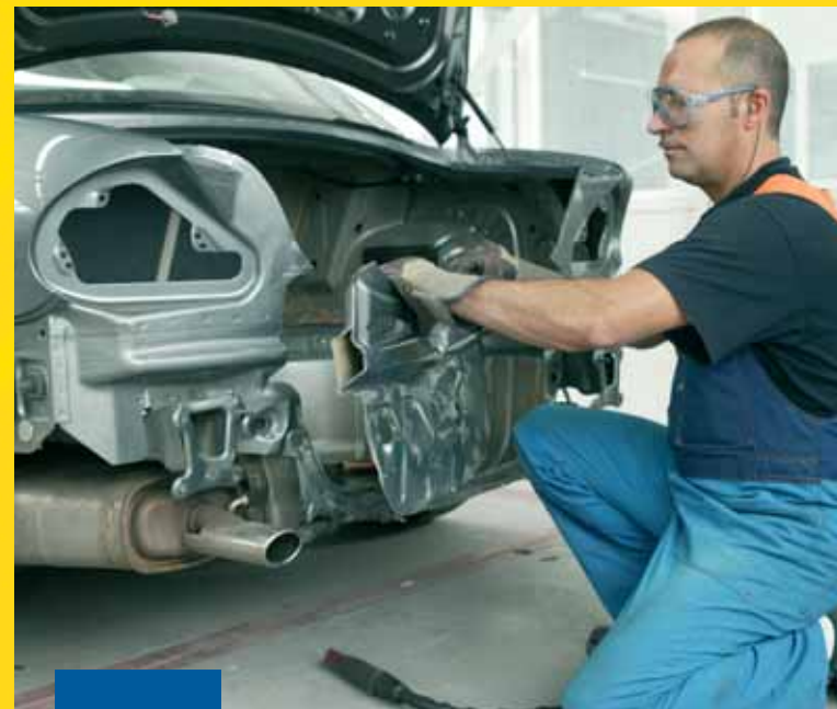
7 Damaged part removal
