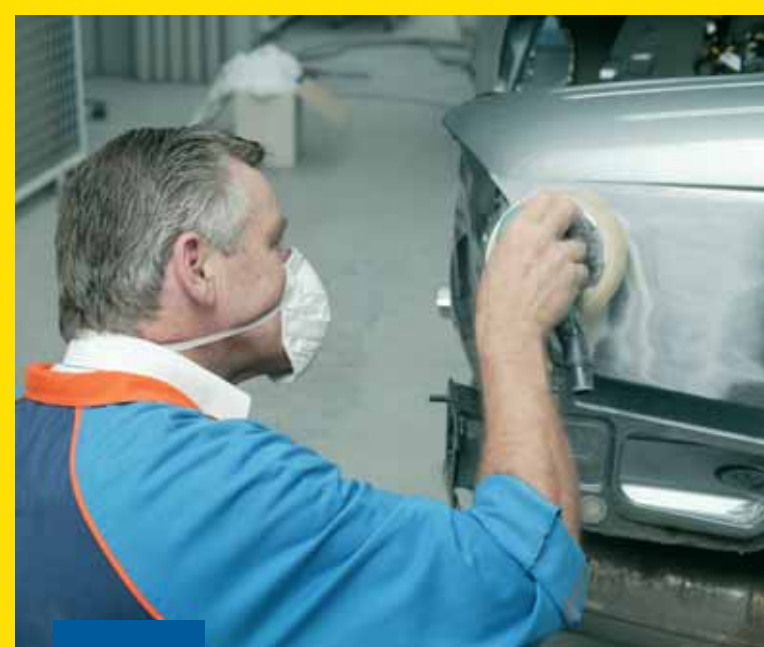
13 Sanding damaged part
